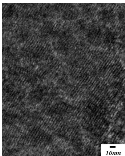
Figure 9. High-resolution TEM image of LC11 crystallized at 125 °C from the isotropic melt and then gradually cooled to ambient temperature.
